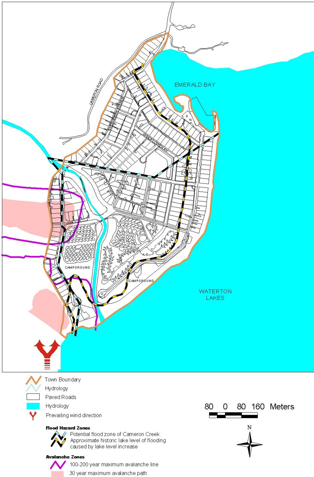
Figure 7.4 Natural hazards in the community of Waterton.
