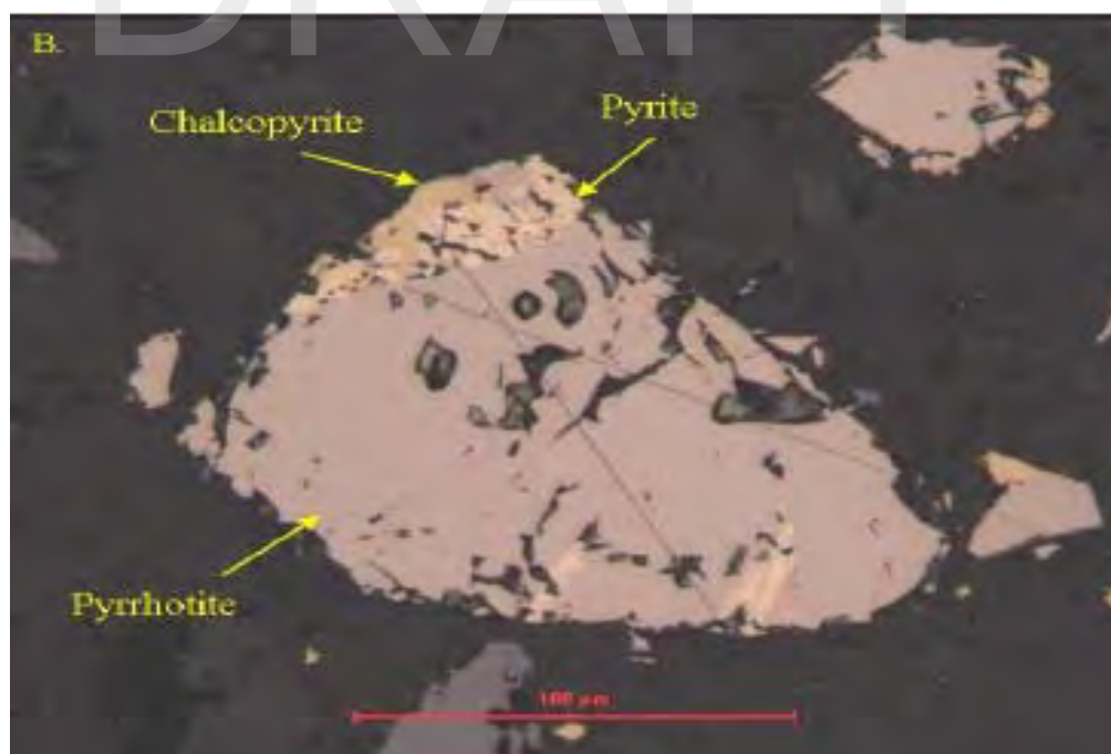
FIGURE B2 Plane-polarized reflected light photomicrograph showing pyrrhotite and pyrite along with chalcopyrite in sample MAR07-16.
