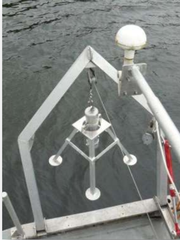
Figure 2. Drop video camera system about to be deployed.
