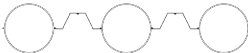
Figure 2. Mur combiné 1219 dia. × 22,225 mm / AZ 26-700
