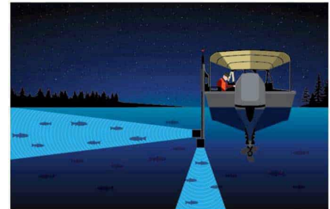
In hydroacoustic surveys, two transducers send sound waves into the water. One of them points down and the other to the side. This allows fish below and to the side of the watercraft to be counted.
