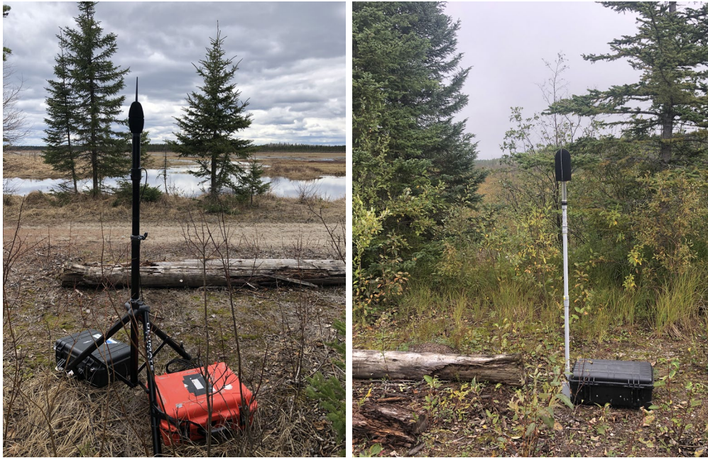
Photograph 4: Noise Monitoring Equipment Deployed at ML4; Leaves-Off Season (left), Leaves-On Season (right)
