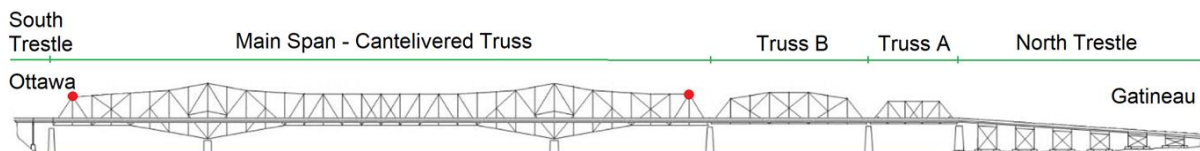
Figure 10-9: Location of pins showing wear issues
