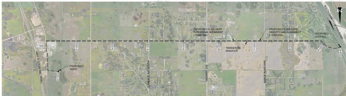
Figure 4.4: Conceptual Forcemain Routing and Discharge
