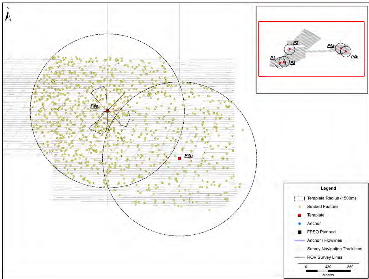
Figure 6-9 Multi-beam echosounder identified hard targets within 1.5 km of proposed drill centres in the eastern Bay du Nord area.
