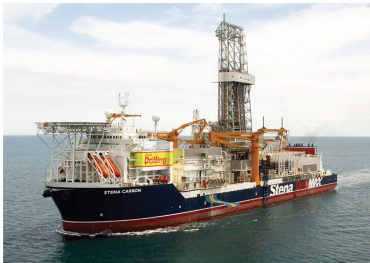
Figure 2-11 Stena Carron - Example of a Drillship
