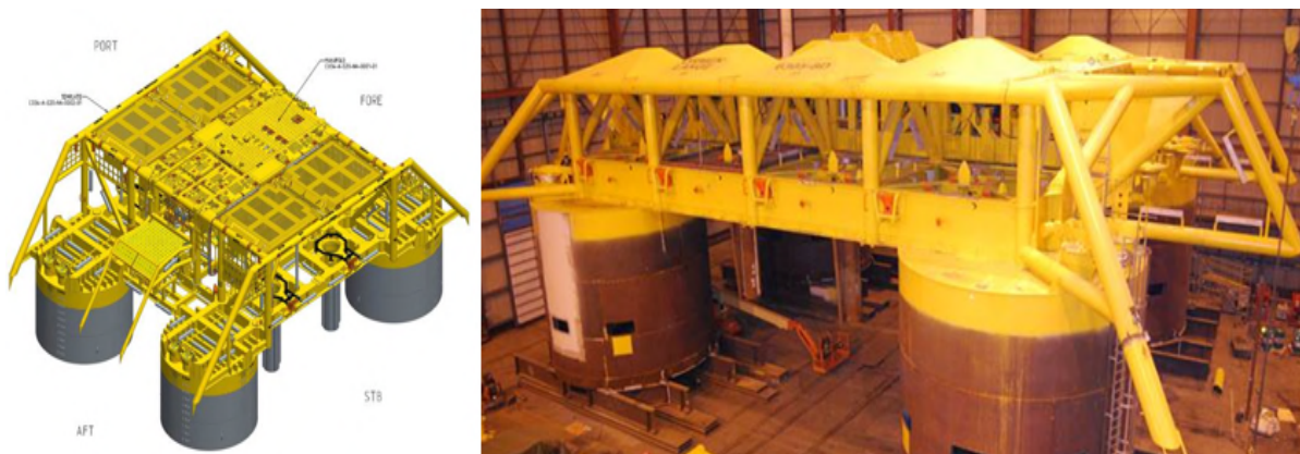
Figure 2-7 Illustration of Representative Subsea Well Templates – 4-slot (left) and 8-slot (right)
