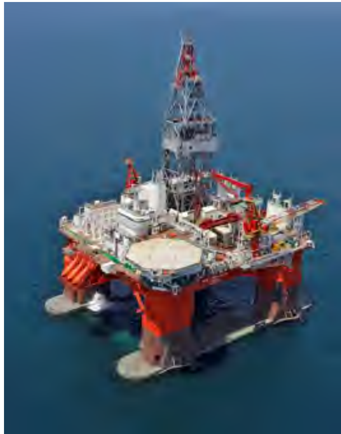
Figure 2-10 West Hercules – Example of a Semi-Submersible
