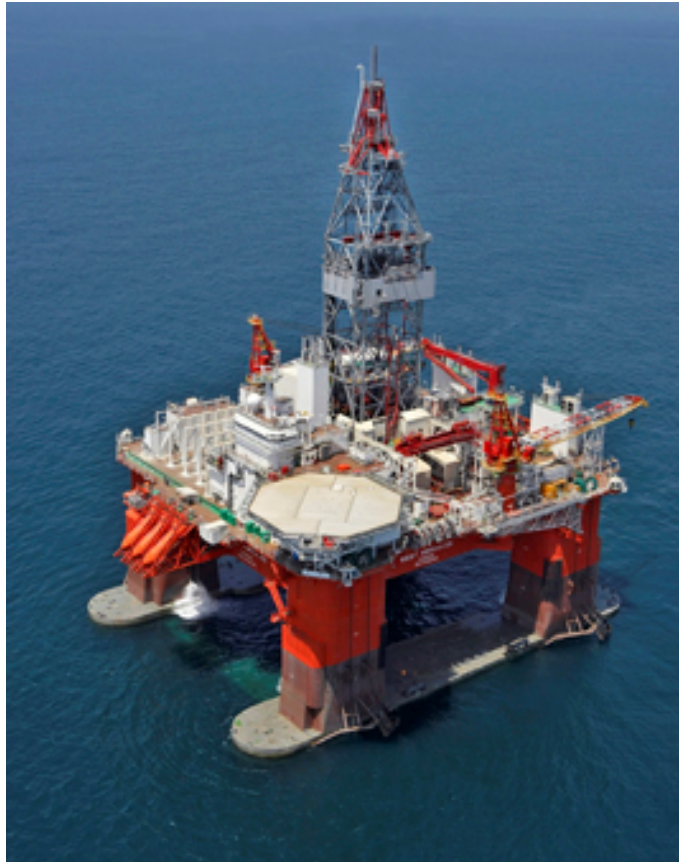
Figure 2-9 West Hercules – Example of a Semi-Submersible
