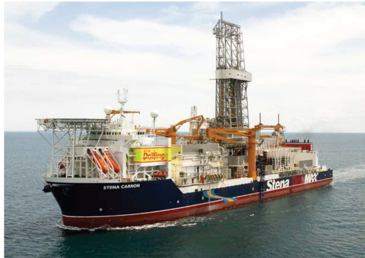
Figure 2-10 Stena Carron - Example of a Drillship
