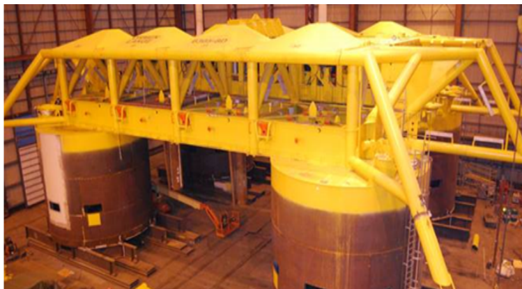
Figure 2-7 Illustration of Representative Subsea Well Templates – four-slot (left) and eight-slot (right)
