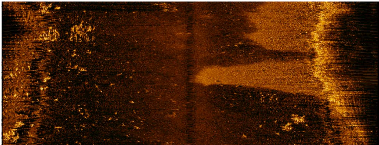
Figure 28. A high-resolution Ping 3DSS-IDX-450 sidescan 'waterfall' image of the transition from cobble, gravel, and boulder substrate to finer sand, silt, clay and mixed gravels in the northeast corner of the West Shore Area. Note the intermittent patches of aquatic vegetation against the dark toned fine substrates.
