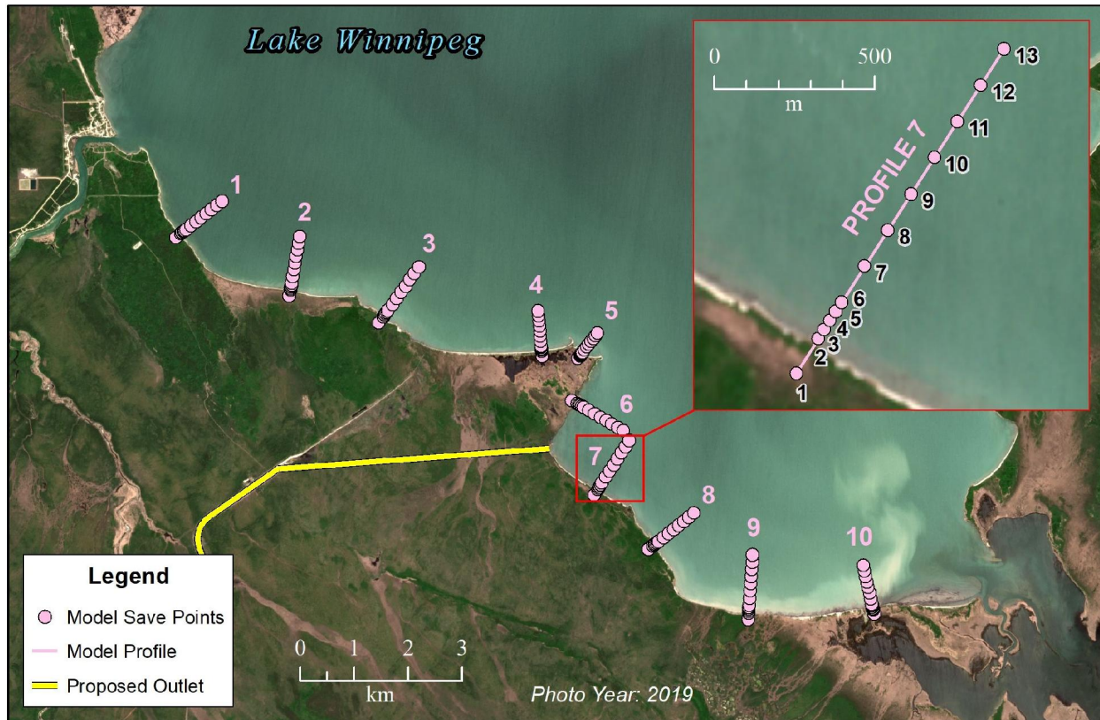
Figure 3.17 Sediment Transport Profiles and the Location of the 13 Profile 7 Save-Points from the MIKE21 Model
