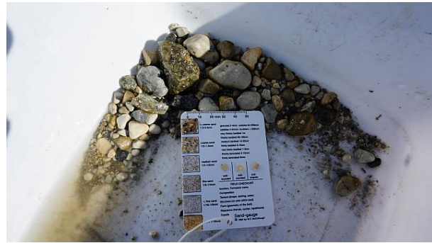
Sand-Gravel at Waterline with Clay
