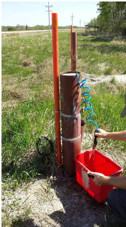
Photo 2. RD15-PW1 – Showing sample purging from tube.
