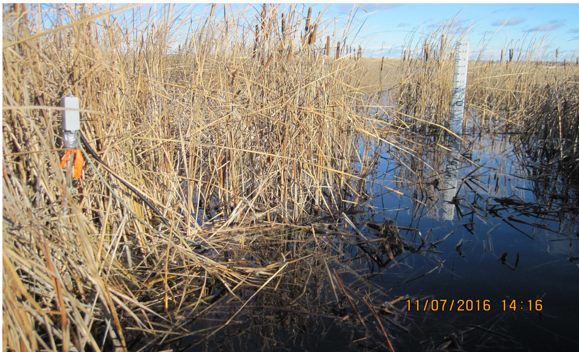
Photo 4. Reed Lake (D3) – Showing staff gauge (right) and transducer (left).
