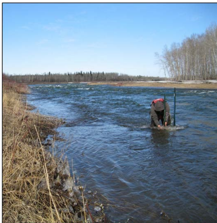
Figure 5-5. Deploying a small drift trap affixed to metal T-bars pounded into the substrate of Buffalo Creek during spring 2012.
