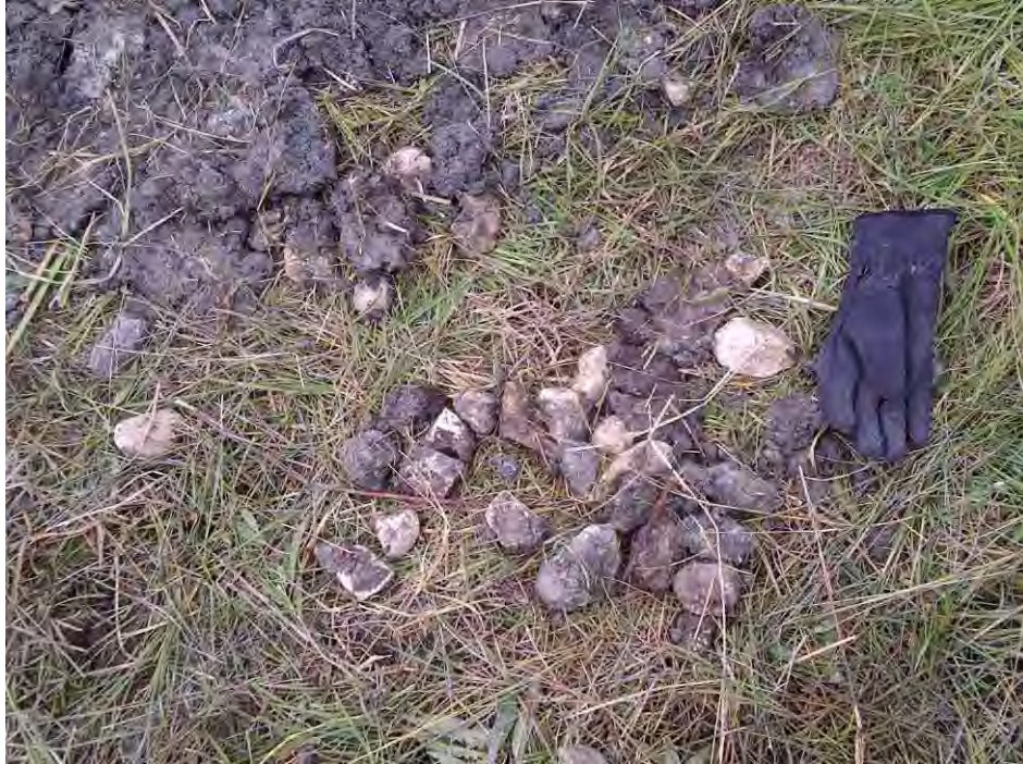
Photo 3 – Material passing 50 mm ø screen
