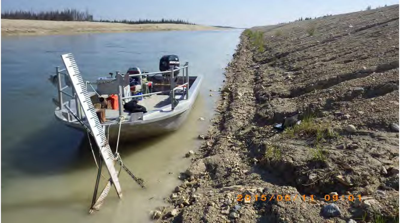
Photo 3. Damaged Gaugeboard at Reach 1 Bench Mark R1-C-A, looking east D/S
