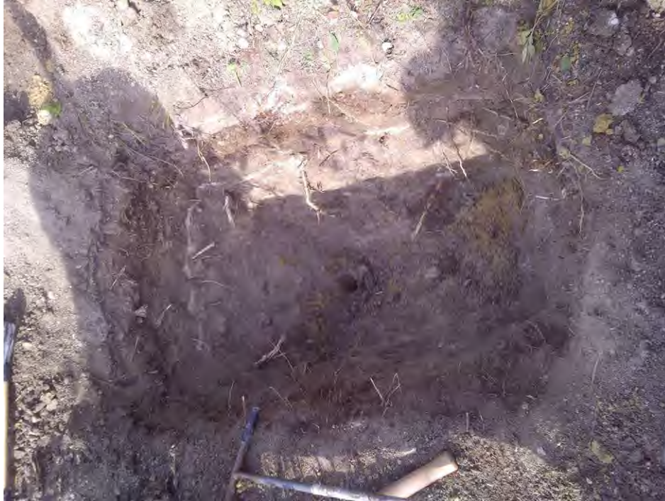
Photo 3 – Base of testpit showing auger hole
