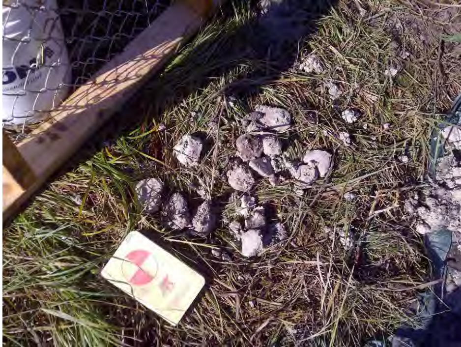
Photo 3 – Gravel <50 mm \varnothing from testpit
