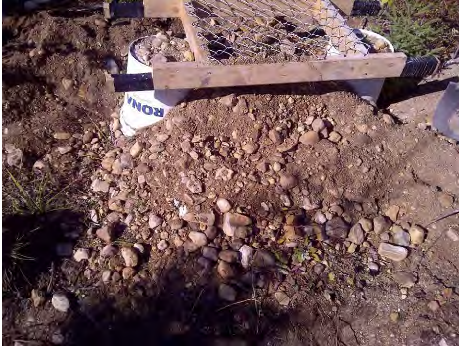
Photo 3 – Screening testpit material
