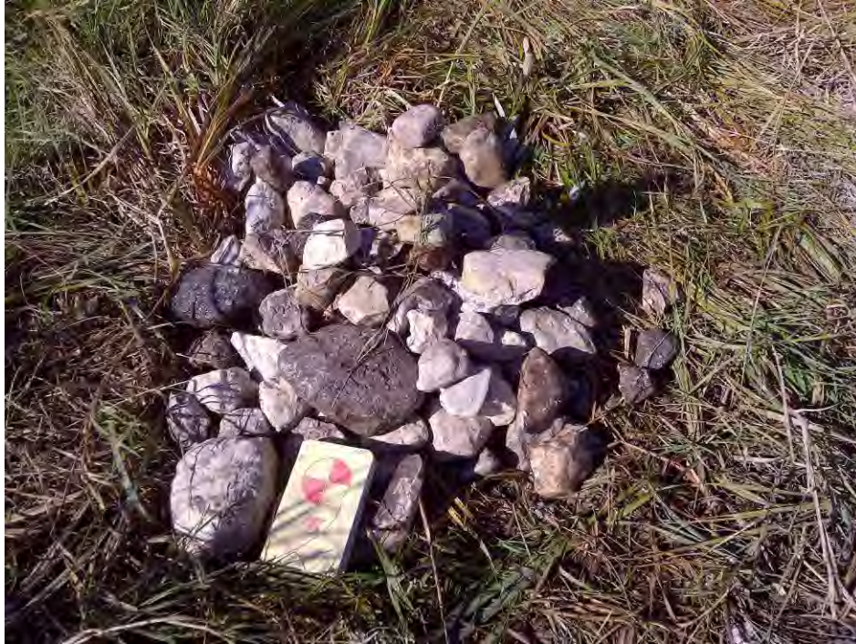
Photo 5 – Coarse material >50 mm \varnothing from testpit
