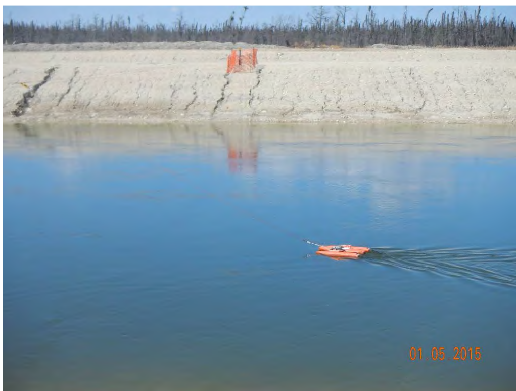
Photo 8. Flow metering with ADCP at Cableway, looking north
