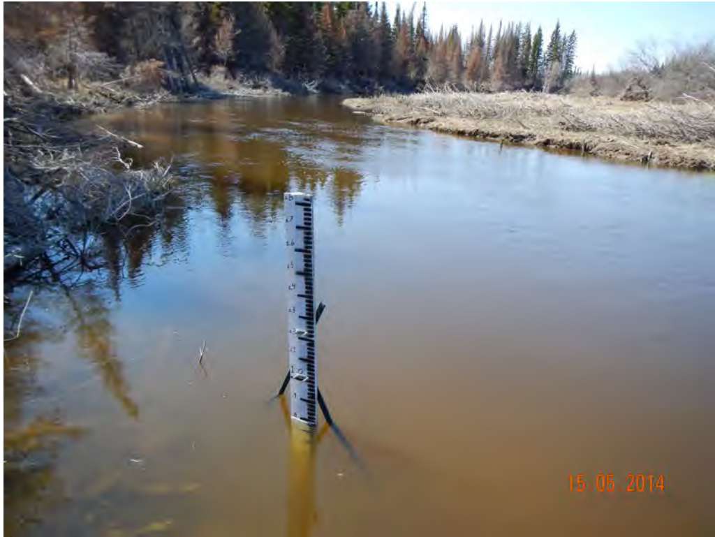
Photo 7. New gauge board installation, Gauge Reading is 0.78 m.
