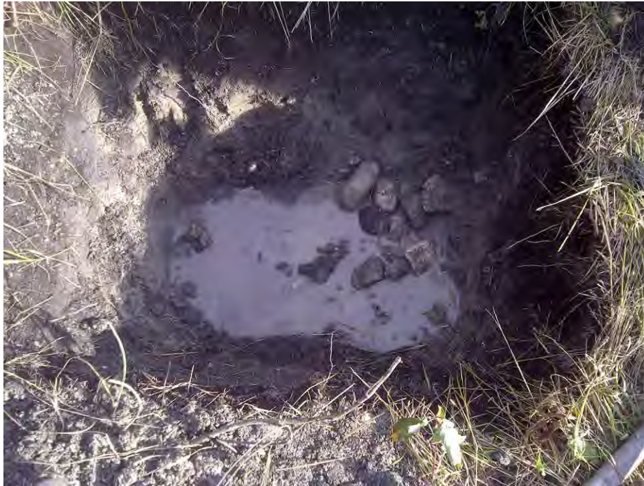
Photo 3 – Coarse material >50 mm \phi from testpit
