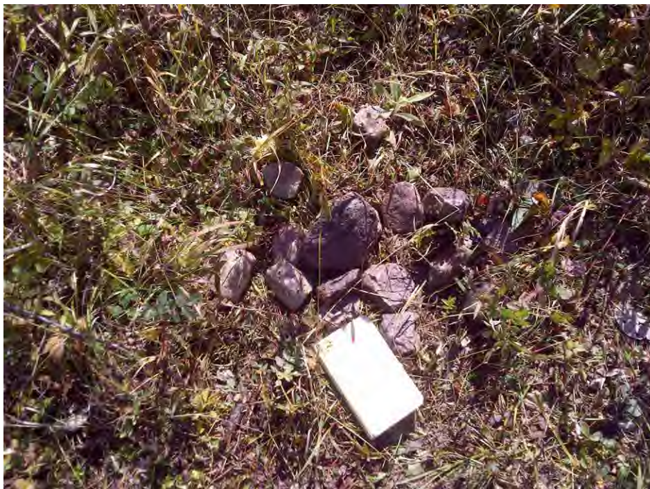
Photo 4 – Coarse material >50 mm ø from testpit
