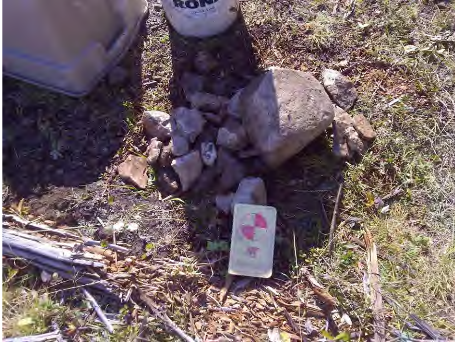
Photo 3 – Coarse material >50 mm ø from testpit
