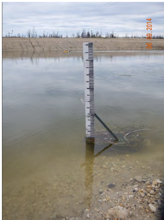
Photo 4: Gauge Board, Reach 1 Cableway, Gauge Reading 0.39 m.
