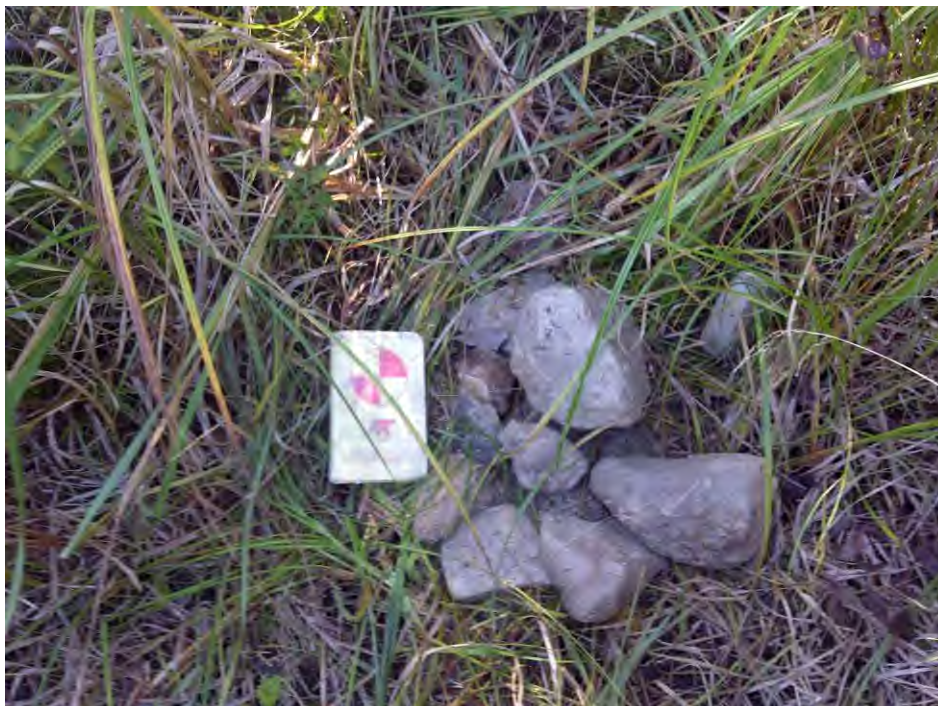
Photo 2 – Coarse material >50 mm ø from testpit
