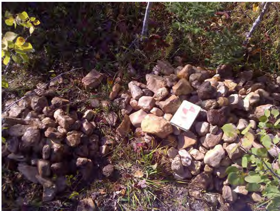
Photo 4 – Coarse material >50 mm ø from testpit
