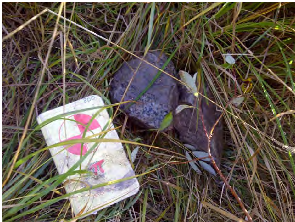
Photo 4 – Coarse material >50 mm ø from testpit
