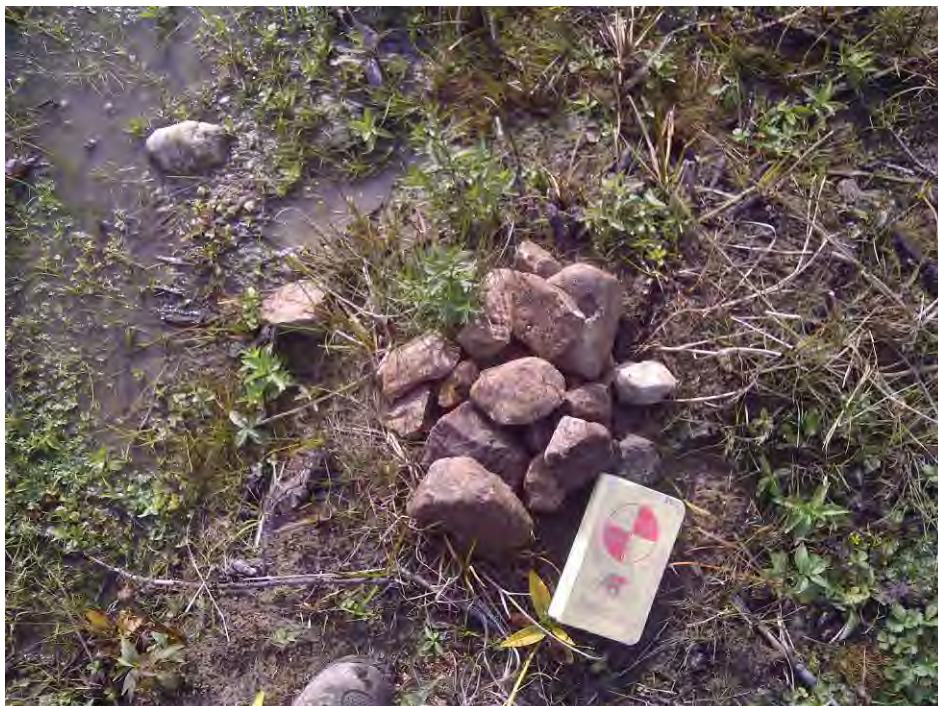
Photo 4 – Coarse material >50 mm ø from testpit
