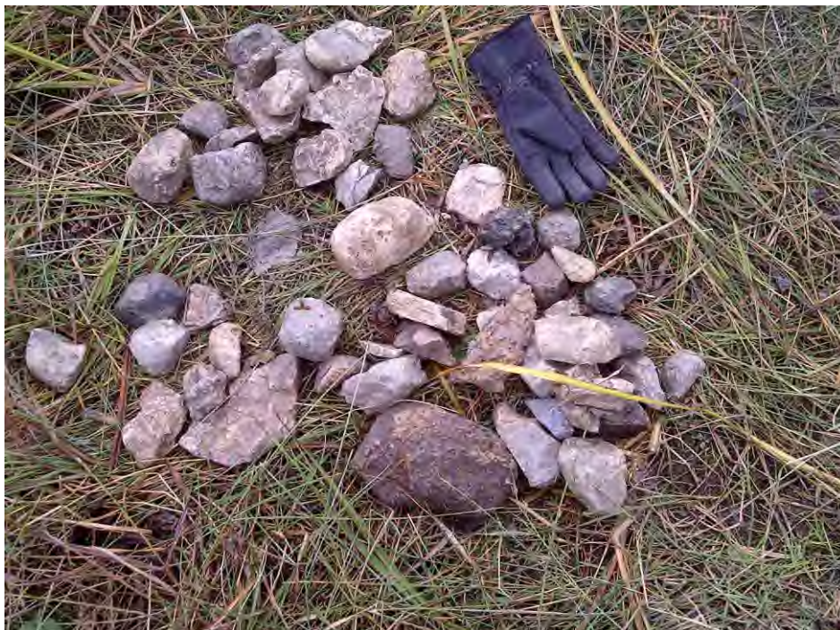
Photo 2 – Coarse material >50 mm ø from testpit
