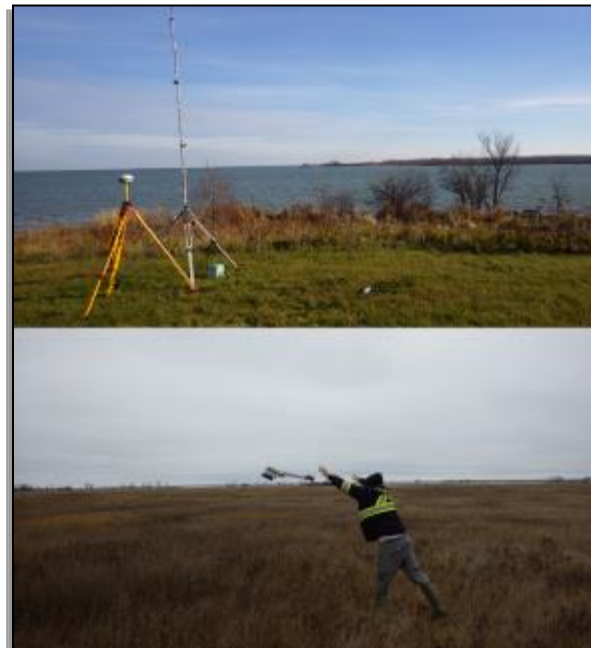
Figure 8. Trimble RX-8 RTK 4 survey equipment (top) and a UAV (eBee drone) launch.
