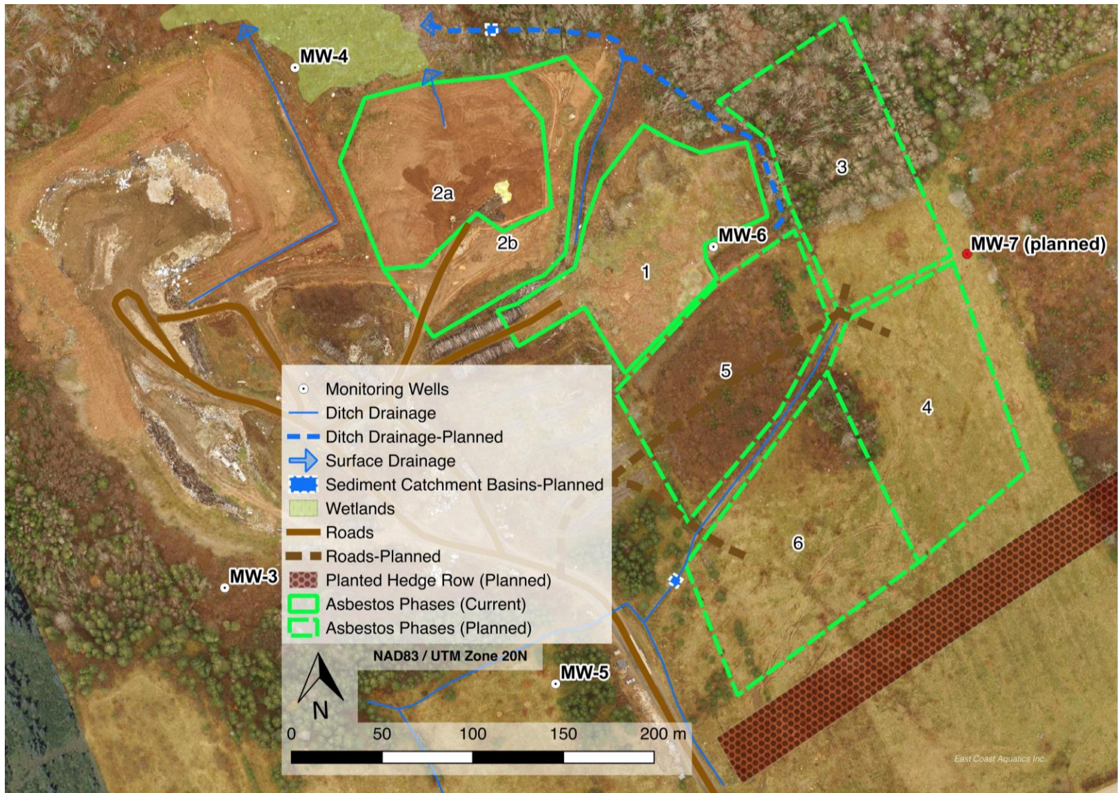
Figure 1: Proposed Arlington Heights asbestos disposal facility site layout indicating the Phased cell locations and well locations. All features currently exist at the site unless otherwise noted. (Based on 2017 drone imagery).
