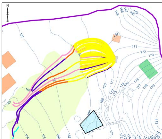
50 m 3 /day discharged to the Exfiltration Gallery
