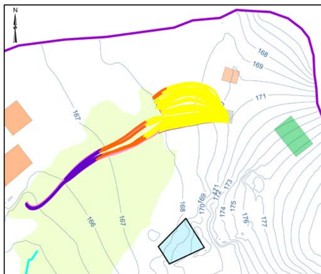
10 m 3 /day discharged to the Exfiltration Gallery
