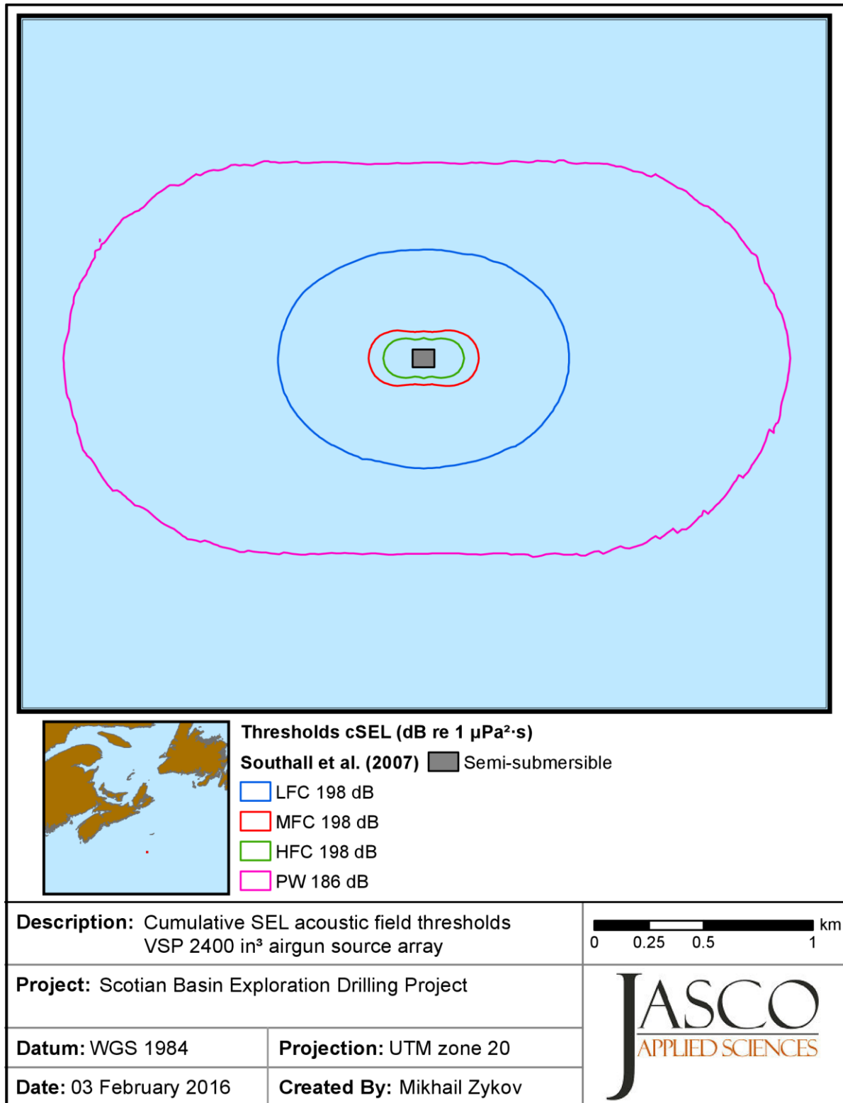
Figure 49. VSP airgun source array: cSEL threshold contours at Site A in winter for the Southall et al. (2007) criteria. Marine mammal hearing groups: LFC–low-frequency cetaceous, MFC–mid-frequency cetaceous, HFC–high-frequency cetaceous, PW–pinnipeds in water.
