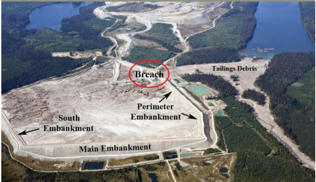
Exhibit 17: Description of Mount Polley dam embankments
