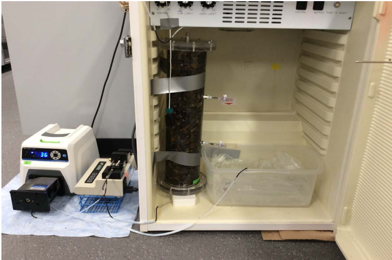
Photograph of Temperature Controlled Column Set Up Grassy Mountain Project, Alberta Geosyntec consultants March 2020 Figure: 2
