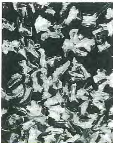
Figure 1: Photomicrograph of silicic glass shards formed from broken bubbles. White zones within some shards are microvesicular frothy areas (magnified 60 x).
