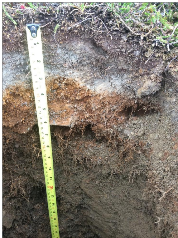
Example of SMU 1a with sandy textures and well developed Ae horizon
