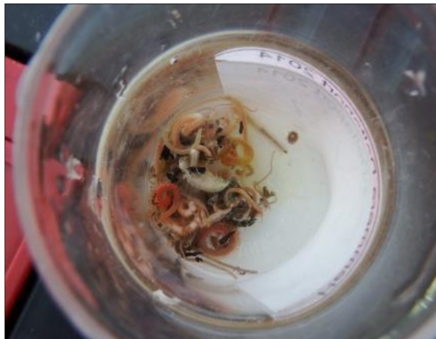
Photo 6 Sieved Macroinvertebrate Samples in a Plastic Jar Prior to Preservation with Formalin
