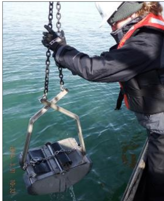
Photo 5 Van Veen Sediment Grab Deployed From a Boat to Collect Subtidal Macroinvertebrates
