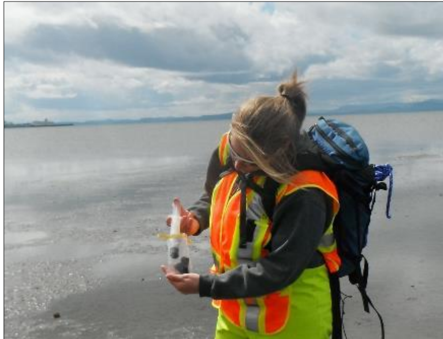
Photo 4 Sediment Core Samples Being Ejected into a Sample Bag and Stored on Ice in the Field
