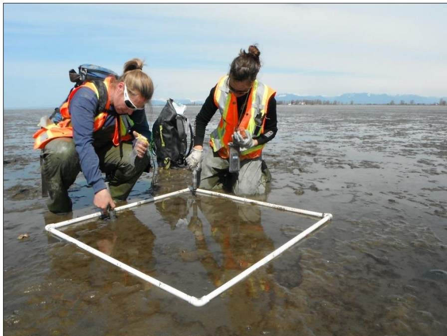
Photo 2 Sampling for Infaunal Using 60 mL Syringes to Extract Sediment Cores at Sturgeon Bank Stratum in Spring 2012
