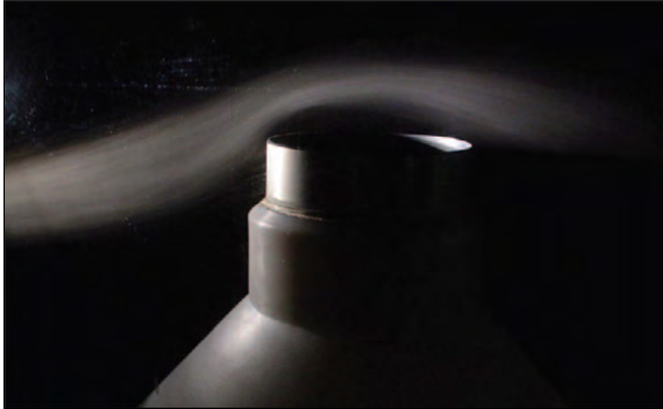
Plate 6.2-1. Laminar wind tunnel airflow around an unshielded precipitation gauge orifice (Rasmussen et al. 2012).
