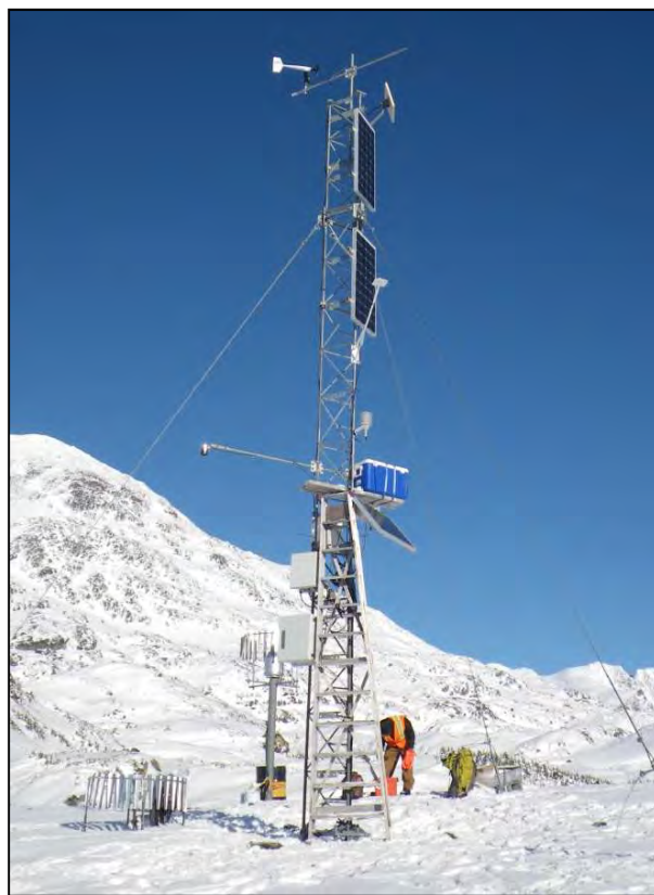
Plate 6.1-1. Brucejack Lake meteorological monitoring station, October 2012.
