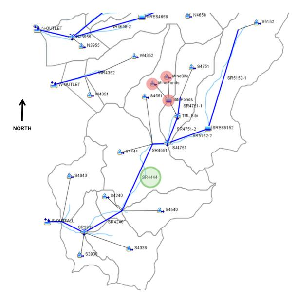
Red – Elements added to simulate minesite developmentGreen – Downstream reach element used for model result comparisons
