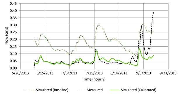
Figure 3-4Measured, baseline simulation, and calibrated simulation results for monitoring station<br/>HS4 (NR4658-2) at the Goliath Gold Project.
