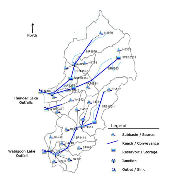
**Figure 3-1** Diagram of the subbasins and model components included in the HEC-HMS basin model for the Goliath Gold Project.
