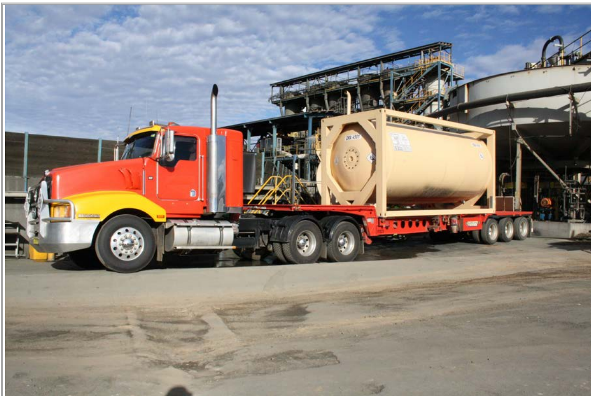
Figure 12.2.1-48: An ISOtainer Carrying Solid Sodium Cyanide Briquettes
