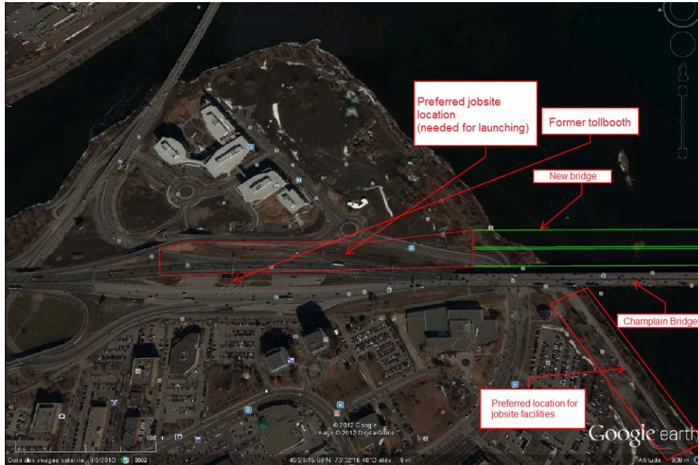
Figure 3 Jobsite location – Nuns' Island
