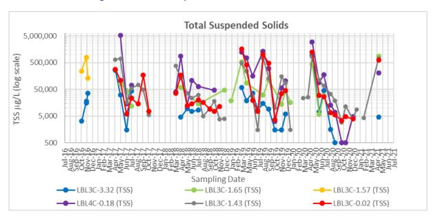
Figure 36a: Total Suspended Solids at L3 Creek Locations
