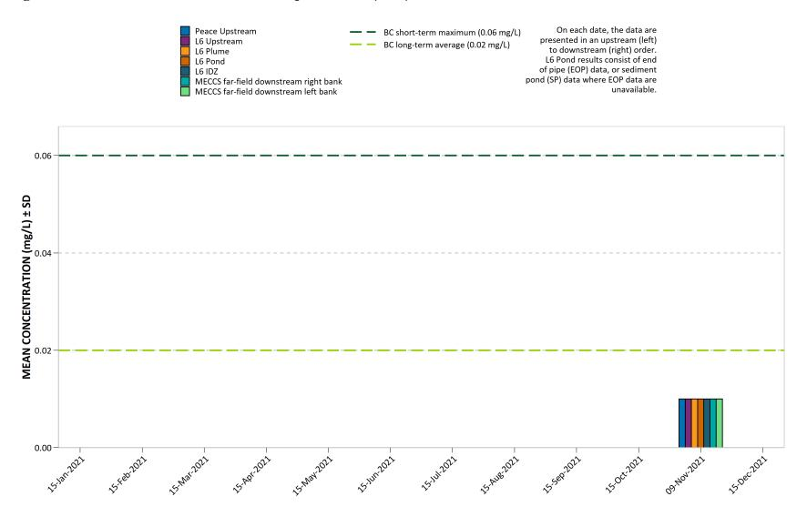
Note: BC WQG for nitrite are chloride dependent, and therefore guidelines depicted in the plot are applicable for Peace River sites only. Based on the range of chloride values observed in the Peace River, the applicable BC Maximum and 30-day guidelines are 0.06 mg/L and 0.02 mg/L, respectively.
