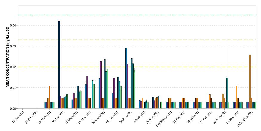
Note: BC WQG for total zinc are hardness dependent. An average Peace River hardness of 106.1 mg/L (based on 26 samples collected between April 2007 – Jan. 2017, BC Hydro 2017) was used in the plot to depict the maximum and 30-day guidelines for ease of interpretation. Sample specific hardness was used to screen individual sample results against guidelines in the data tables (Appendix A).
