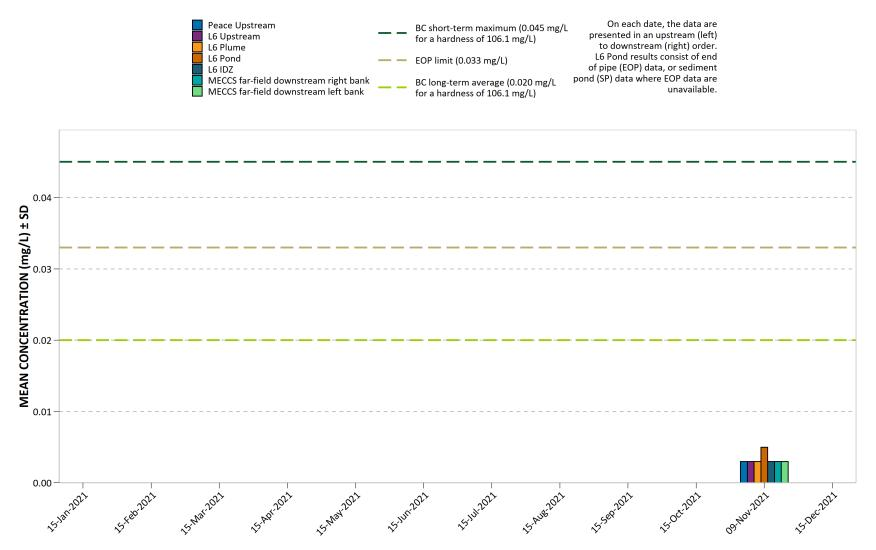
Note: BC WQG for total zinc is hardness dependent. An average Peace River hardness of 106.1 mg/L (based on 26 samples collected between April 2007 – Jan. 2017, BC Hydro 2017) was used in the plot to depict the maximum and 30-day guidelines for ease of interpretation. Sample specific hardness was used to screen individual sample results against guidelines in the data tables (Appendix A).
