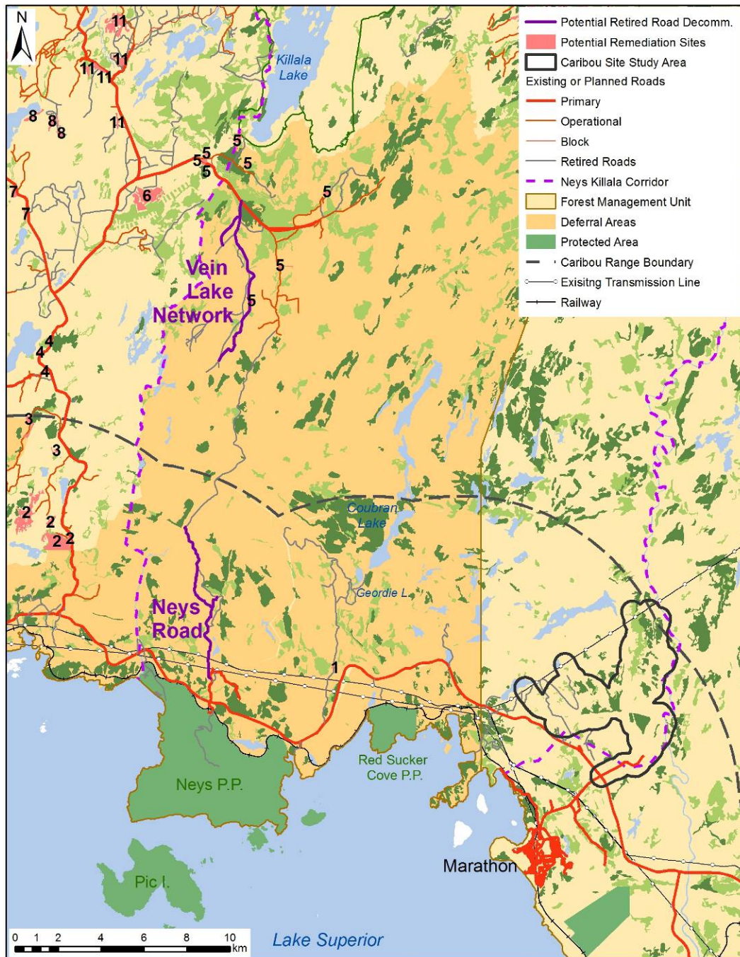
Figure 18. Location of Neys Road and Vein Lake road network, two "retired" roads with potential for decommissioning.
