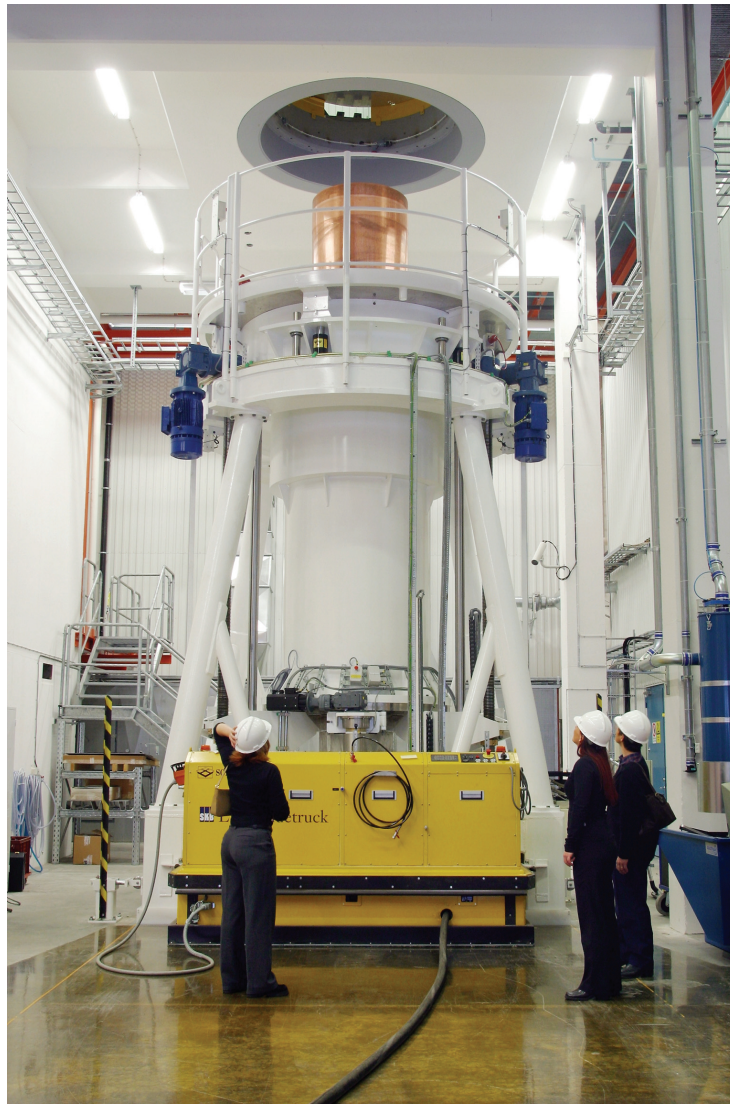
Figure 4-4: Shielded Frame and Air-cushion Transporter
