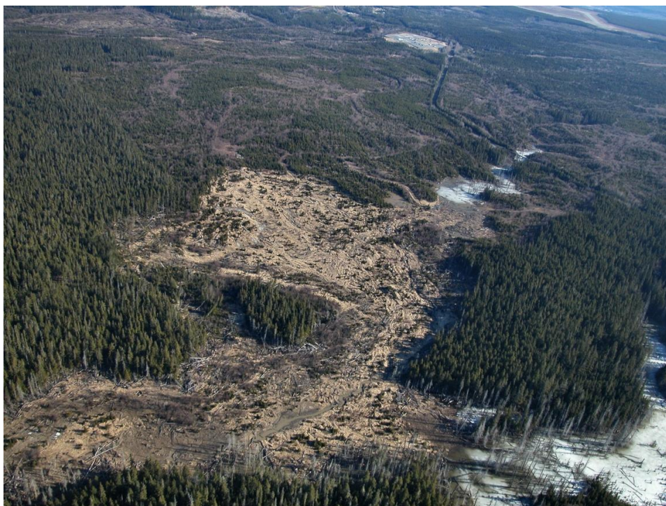
Figure 14: The Mink Creek flow slide rapidly retrogressed along a slope of about 3°, approximately 23 ha flowed into Mink Creek, extending downstream for 1 km.
