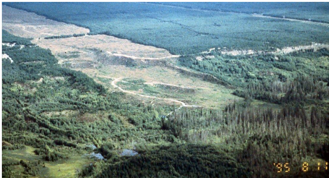
Figure 15: Foreslope of the Onion Lake Flats (fan-delta) to the east of Cecil Creek. Roads follow arcuate ridges that outline prehistoric flow slides. The ridges are visible in the clearcut (photo centre) and in the area reforested (photo centre-left).
